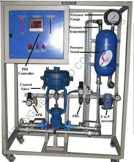
The Air Pressure Control Trainer (PCST - 03 B) is the system which outlines the basics of Closed Loop Air Pressure Control and various aspects related to it.
