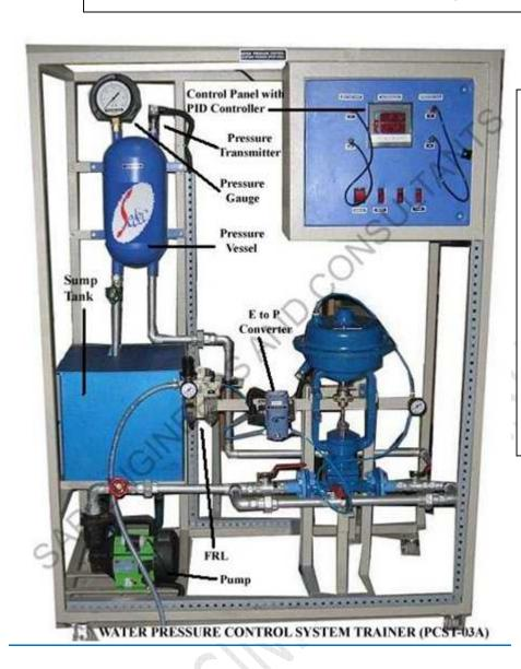
The Water Pressure Control Trainer (PCST - 03 A) is the system, which outlines the basics of Closed Loop Water Pressure Control and various aspects related to it
